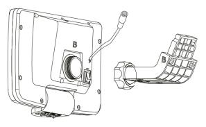
Attach the bracket marked "B" to the back of the lamp (also marked "B") and tighten the hinge by hand.
