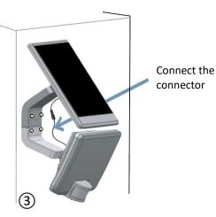
Connect the solar panel to the luminaire
