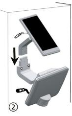
Slide the solar panel with bracket "B" onto bracket "A" on the luminaire and secure with
